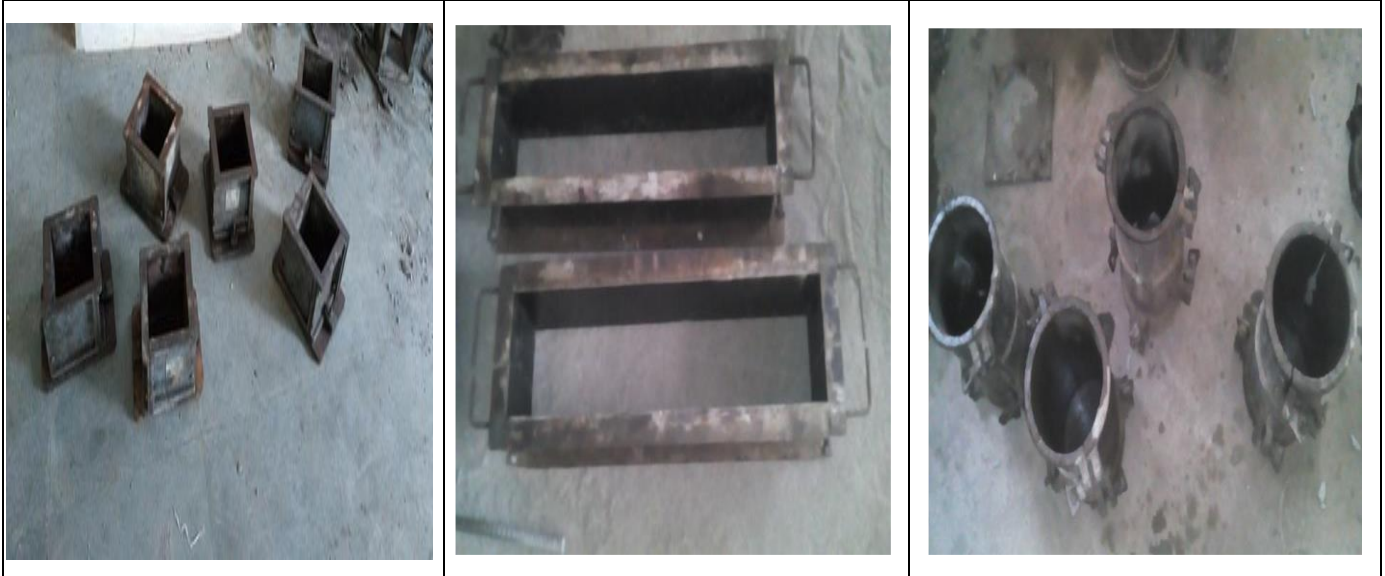
Fig.1. Cubes, Prisms and cylinders Molds.
